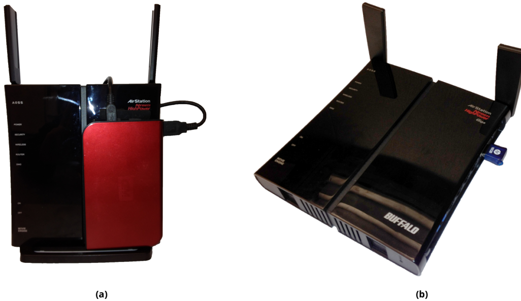
Figure 4: Open Infrastructure testbed devices: Buffalo WZR-HP-G300NH (a) 3.5" hard drive , (b)16GB USB Flash.
